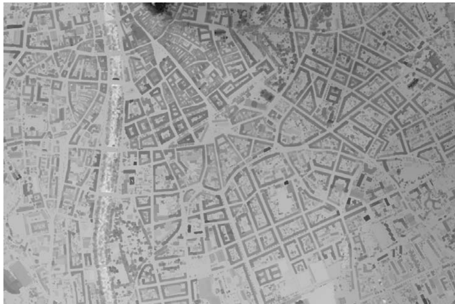
Figure 4. A dense height image with a GSD (ground sampling distance) of 30cm for the inner city of Graz is calculated fully automatically from oriented aerial images.
