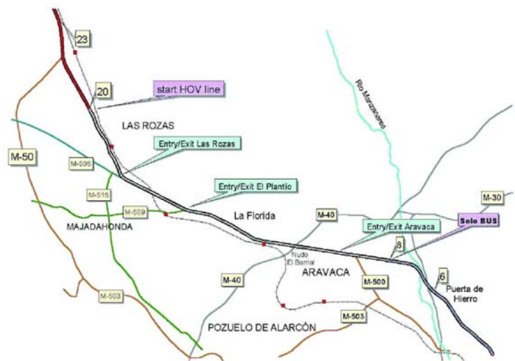
Figure 5: Bus/HOV lane, stretches and access points (Monzón, et al. 2003)
