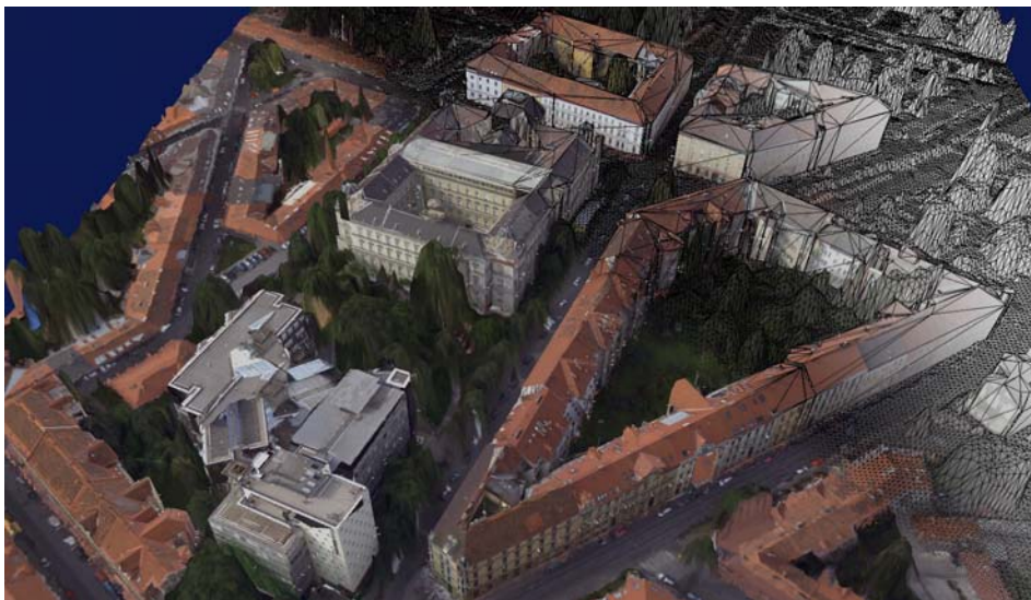
Figure 6: 3D city model of a small area in Graz. Additionally to the geometry and texture information, the semantic of single objects (building block, tree, street, water region, ...) is known as well.
