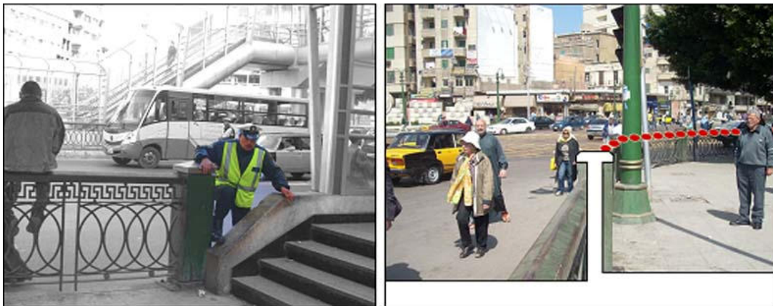
Fig. 7: Al Horreyah Avenues' sidewalks that have long block barriers which prevent pedestrians from joining the same platform
