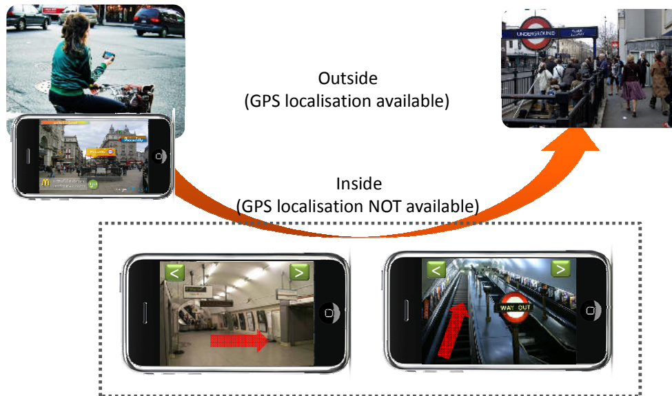
Fig. 6: a viable hybrid routing strategy for i-Tour based on full map based (in outdoor contexts) and landmark-based guiding (in indoor context with no localisation)
