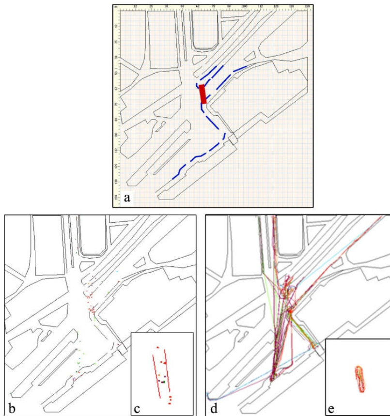
Fig. 14: (a) Shows the bridges' virtual new location on the top view through Simwalk Draw software as a proposed design. (b,c) image shows agents scenario with the proposed bridge location that gives more chances to join the upper level using the pedestrian bridge. (d,e) image shows the results presented in trails
