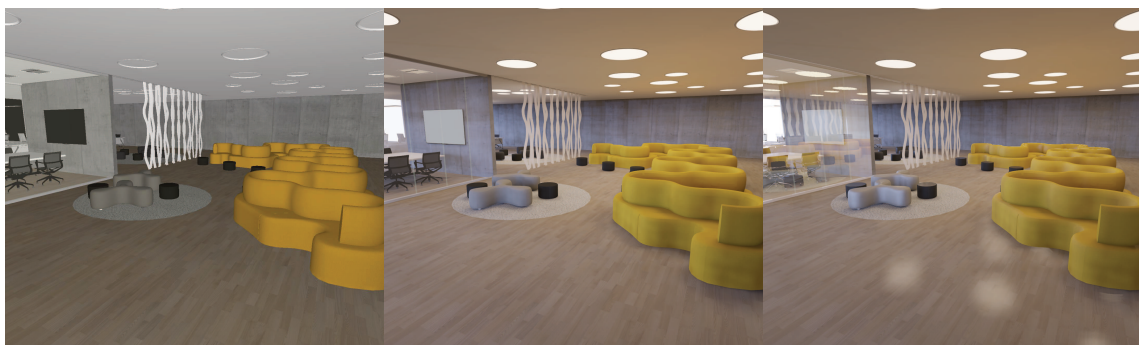
Fig. 3: Various renderings of the same scene. Left: Abstract material shading. Middle: Illumination values applied to material model. Right: Illuminated scene inclusive view dependent material effects.
