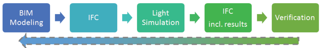
Fig. 4: The workflow concept and its components. Based on the BIM data, an IFC file is generated. The IFC file is analyzed, and the semantic data is used to enrich material properties, place measurement surfaces according to industry norms, and load photometric light profiles. After the physically correct light simulation, the results are stored, and the verification process is performed. In the future, these results will be made accessible to the original BIM again (via IFC).
