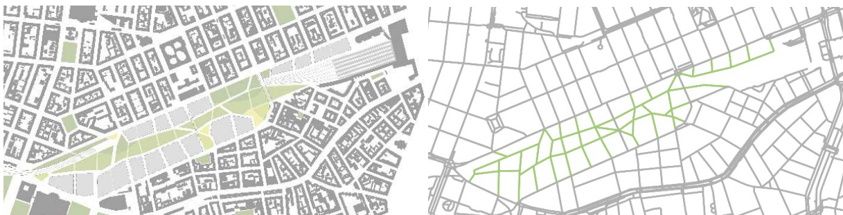
Fig 8: left: Site plan, the block size provides frequent route choice and the park provides cooling and space for recreation; right: The pedestrian network provides optimal connectivity considering the topography and remaining train connection © Tobisch
