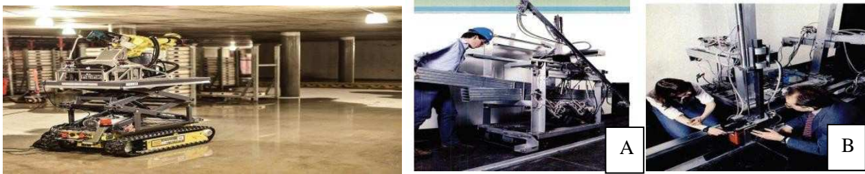
Fig. 26 (left): drilling robot (nLink, 2016). Fig. 27 (right): A) studbot system B) trackbot systems (Bock, 2016)
