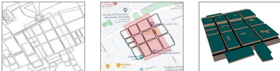
Fig. 3: The development of work on building the case study. Left: autocad site map, Middle: Google site map, Right: Revit 3d model as masses
