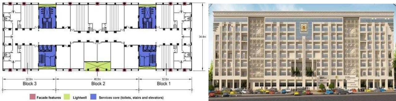
Fig. 28 (left): Building repeated floor plan showing zones (Researchers, 2021). Fig. 29 (right): Building main façade visualization (Youssri Azzam, 2019).
