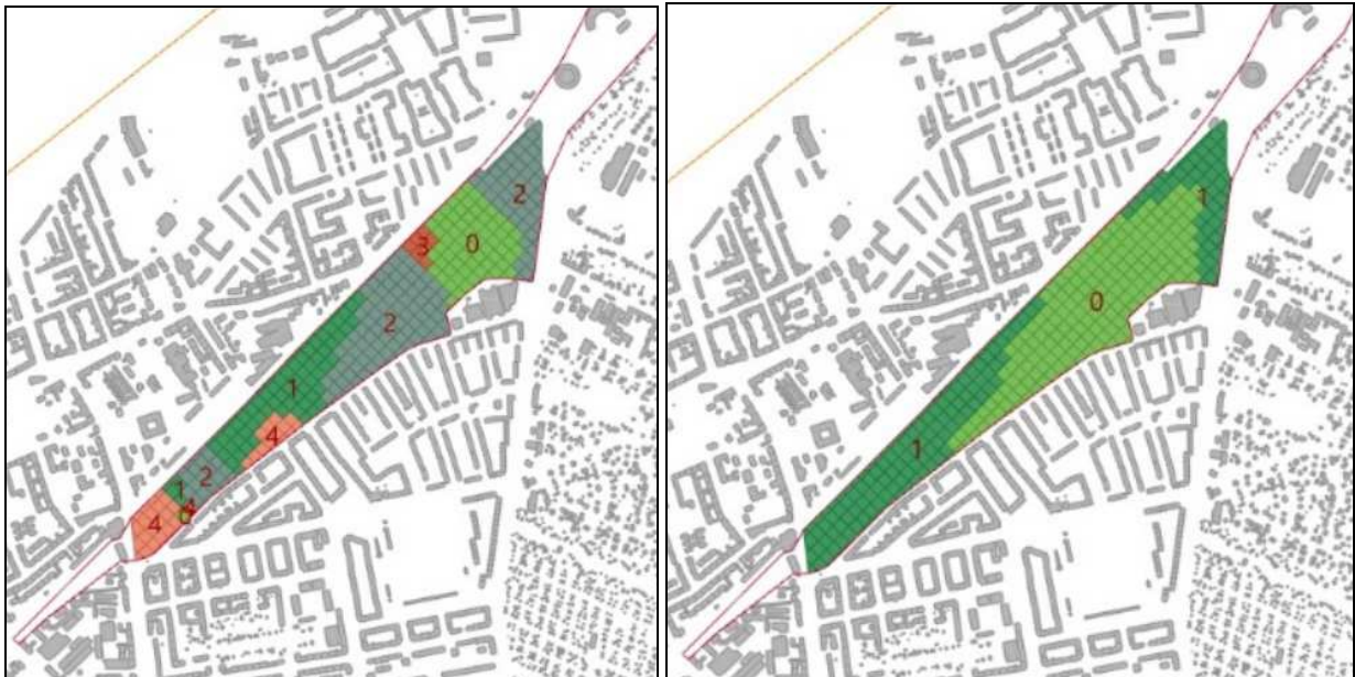
Fig. 7 (left): Suggested land use by ANN for the ground floor: 0 – local amenities, grocery, 1 – no specific ground floor use, 2 – commercial (work), 3 – educational amenities, 4 – commercial (retail). Fig. 8 (right): Suggested land use by ANN for upper floors: 0 – residential, 1 – commercial.
