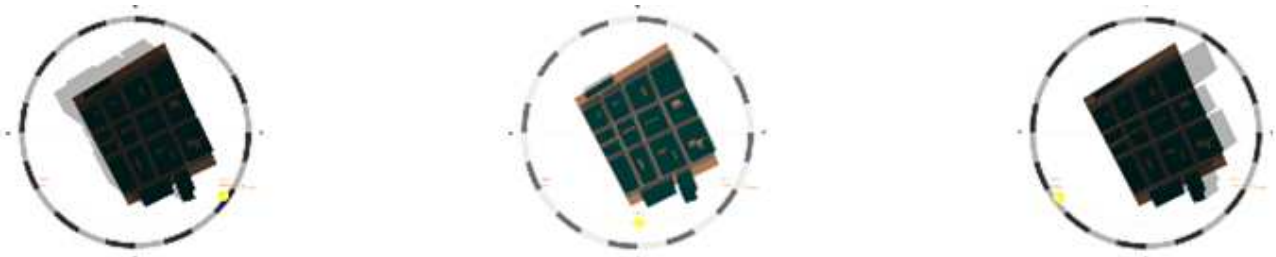
Fig.14: Site plan Shade and Shadow in winter. Left: 8 o'clock, Middle: 12 o'clock, Right: 16 o'clock
