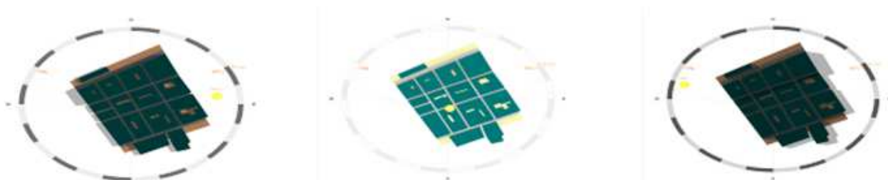
Fig. 5: Site plan Shade and Shadow in summer. Left: 8 o'clock, Middle: 12 o'clock, Right: 17 o'clock
