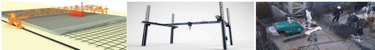
Fig. 8 (left): concrete levelling robot (Kajima, 2016). Fig. 9 (middle): COBOD 3D printer (Peri, 2021). Fig. 10 (right): Vertical reinforcement robot (Fujita, 2016).
